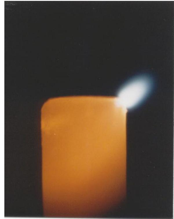
The current is localized in a region occupying a small fraction of the surface (cathode spot); the **spot mode**.
